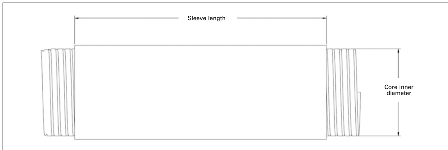
Figure 3. EZ Seal sleeve and core dimensions
