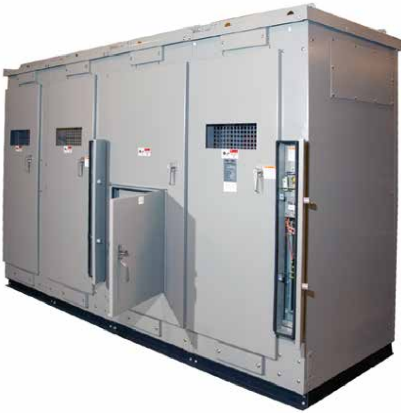
Figure 1. Type ME Motor Operators are mounted in the switchgear stile, adjacent to the compartment door opening and allowing the enclosure width to remain at only 36 inches. Federal Pacific's source-transfer relay is mounted on the switchgear in a separate low-voltage enclosure. As pictured above, the SEL-451 relay is mounted on the compartment door of the second bay from right.
