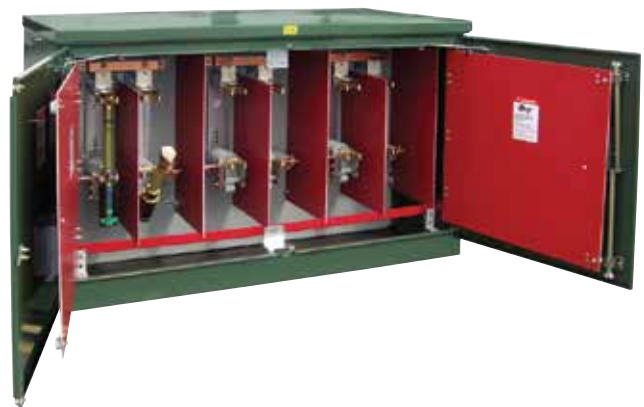
Figure 4. The FUSE compartment is pictured with the barriers secured open and showing one set of two fuses on the left phase – one fuse is latched closed and one fuse is shown in the disconnect position. The fuse mountings are non-loadbreak so the elbow has to be used to break the load current, de-energizing the circuit, before disconnecting the fuse.
