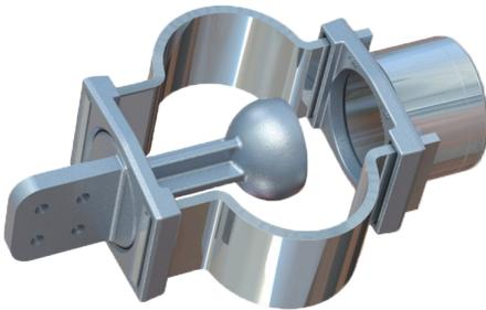
An economical connector making a permanent union between a terminal and a tubular bus, the swage expansion terminal is made of a lightweight and corrosion-resistant aluminum that compensates for temperature variations and thus protects equipment bushings, switch gear, and insulators from expanding or contracting bus pressures.
