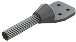
A reliable and economical connector for joining a cable to a flat bar bus, the type WCP cast of a lightweight and corrosion resistant aluminum alloy makes a permanent connection. Side formed NEMA pads are standard.
