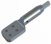
The A1C aluminum compression terminals for connecting aluminum cable to a flat pad utilizes a standard hex die and can be installed with a single crimp. The crimping die sizes are clearly marked for ease of installation.
