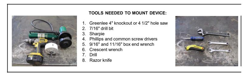
**STEP 1:** Determine the best location to mount device. Mark and cut 4 1/2" hole.
